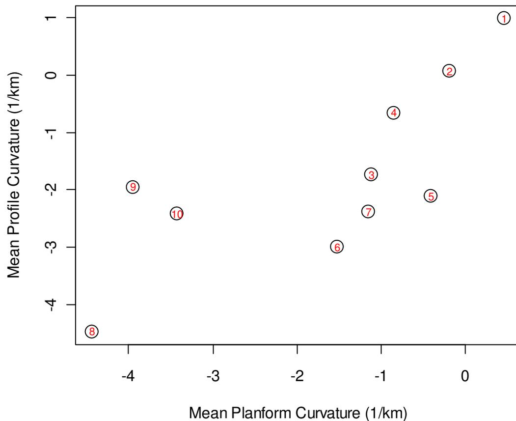
Figure 3. Slope curvature (profile and planform) for each of the 10 study swales. Negative values of planform curvature correspond to convergent slopes (concave on the contour), while negative values of profile curvature correspond to slopes with accelerating flow (concave in the direction of the slope gradient).
