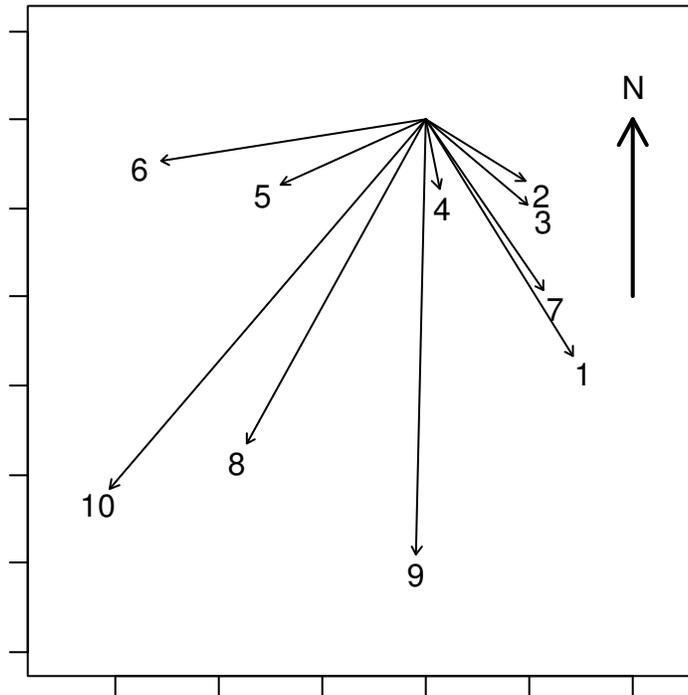
Figure 1. Swale gradients. The directions of the vectors represent aspect, the lengths are proportional to slope steepness, and the numbers are the site IDs.
