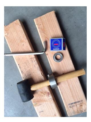
Put new bearing into holder and reattached. Grease with High temperature FOOD GRADE GREASE ONLY. Every month apply some grease to front bearing. Back bearing only needs greased every couple months unless using roaster daily.
