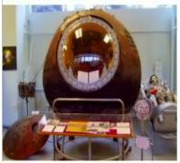
The craft consisted of a spherical descent module (diameter 2.3 meters, mass 2.46 tons), which housed a cosmonaut, instruments, escape system, & a conical instrument module(mass 2.27 tons, 2.25 m long, 2.43 m wide). Holding propellant & an engine system. On reentry, the cosmonaut did eiect from the craft at about 7,000 m descend via parachute. The capsule would land separately.
