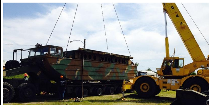
Employees of the Logistics Readiness Center and TACOM load the Mobile Assault Bridge onto a Heavy Equipment Transporter for movement to the paint shop.
