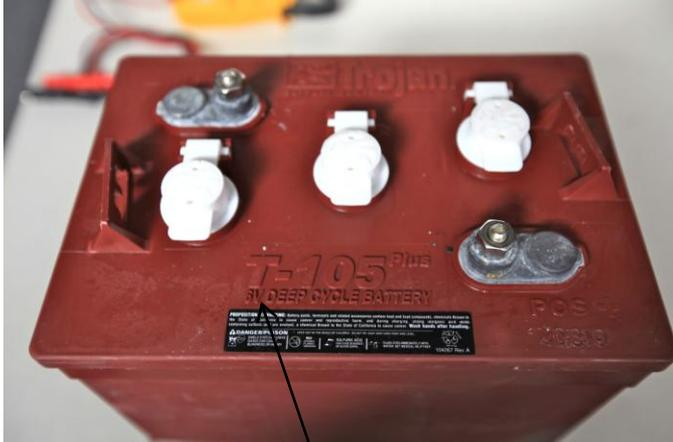
The Trojan six volt T-105 battery will put out 75 amps for 115 minutes. This battery would be considered a 225 amp rated.
