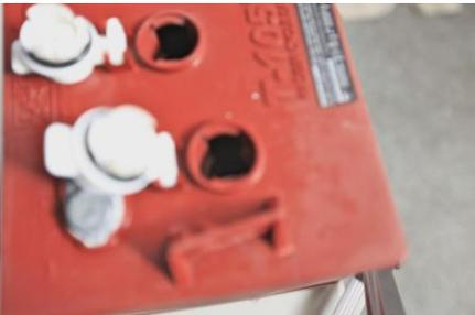
When you fill your battery with water DO NOT FILL TO TOP! Look inside for the plates and fill to ½ inch over the plates AFTER CHARGING.
