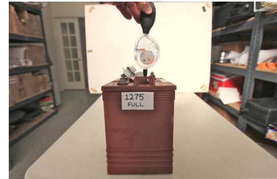
This type of battery is designed to be charged and discharged hundreds of times. An automobile battery cannot be cycled like a golf cart battery. The alternator in a car provides the electricity once the engine starts running. The car battery is designed only to start the engine.
