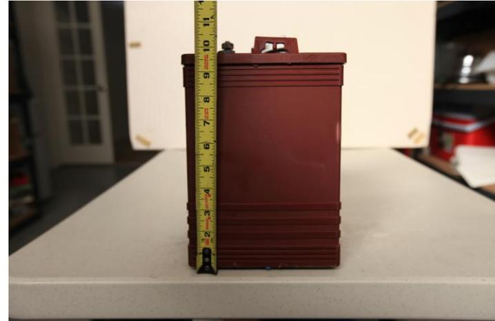
Deep cycle batteries have a reservoir of space near the bottom that makes them taller than starting batteries. The plates inside are thicker than auto batteries too. Deep cycle batteries will charge back up from being discharged without harming permanently. The small amount of oxide that sloughs off the plate lands in the reservoir space and does not come into contact with the plates, keeping them from shorting out. Since the plates are thick they can survive many cycles before they fail.
