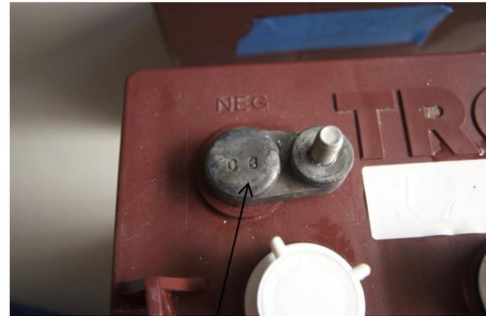
Trojan stamps the date the battery was made into the top of the negative post. The letter represents the month and the number equals the year. This battery was made in March of 2003
