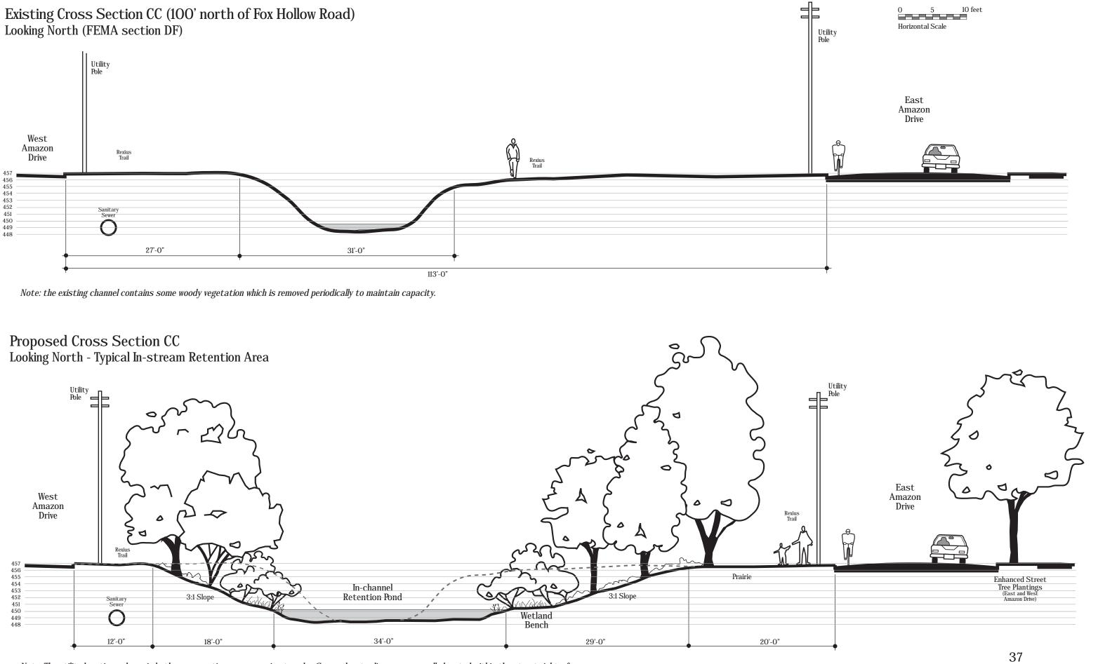
Note: The utility locations shown in both cross sections are appoximate only. Gas and water lines are generally located within the street right-of-way.
