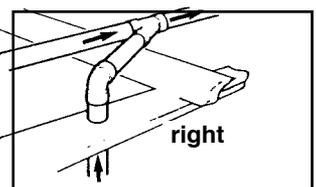
to the effects of gravity. The result will be a pile of dirt at the base of the inlet valve every time it is opened. To avoid this situation the following techniques should be used.
