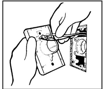
trimmed mounting plate. Bare 1 inch of both wire leads and wrap them around the lugs on the back of the valve in a clockwise direction. Tighten the lugs with a Philips screwdriver.
