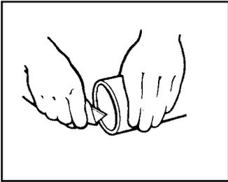
Before cementing both the tubing and the fitting must be free of PVC burrs, dirt and grime. The components should be wiped with a clean cloth if necessary. Cement should be applied to the tubing only as cement applied to the fitting will be pushed ahead and create a rough bead on the inside of the fitting.
