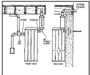
\*\*Vacuums must breathe ... do not enclose. If the unit is to be located in a closet or utility room it must be vented. Louvered doors fulfill this purpose. A muffler can, of course, be used to minimize noise.
