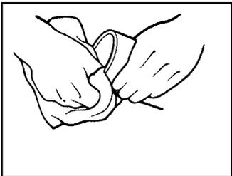
This bead will reduce airflow and could cause a clog. The tubing should be inserted all the way into the fitting and twisted a quarter turn to evenly distribute the cement. All excess cement should be removed with a rag. The glue should be allowed several hours to set before the vacuum system is used.
