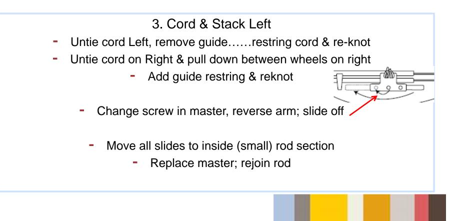
Converting a 1 Way Traverse to a 2 Way
