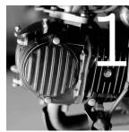
After removing the two bolts, remove the OEM timing gear cover.
