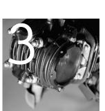
Screw in the top bolt by hand until it is snug, then screw in the bottom bolt the same way. Use a wrench to tighten the two bolts. This assures your new cover goes in straight and will not leak. The new cover should be tight against the motor housing when you are done.
