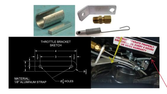
RETURN SPRING RIVETED TO GAS TANK BRACKET
