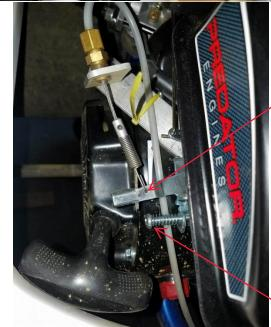
Drill lever to accept the briggs throttle clevis.
