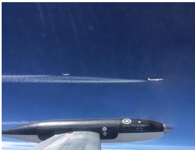
Photo taken during International flight tests under IFAR to study the effects on emissions and contrail formation of burning alternative fuel in jet engines
