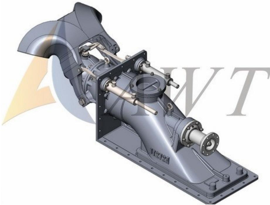
\*Rear Thordon bearing \*Greased Front thrust bearing
