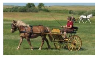
Shafts, 77" long -- Shaft width at cart end, 38" -- Shaft width at narrowest, 27" -- Width of cart floor, 40" Wheel diameter, 36"
