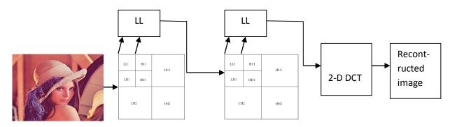
Fig.4: Hybrid (DCT-DWT) image compression
