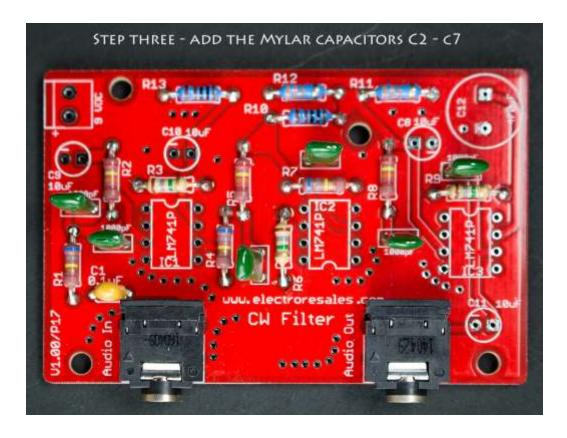
This photo illustrates the Mylar capacitors being close mounted to the PCB
