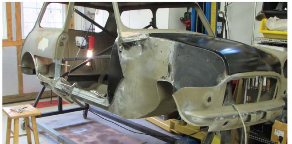
We fabricated a new rear lower 1/4 panel from the old door skin we replaced.
