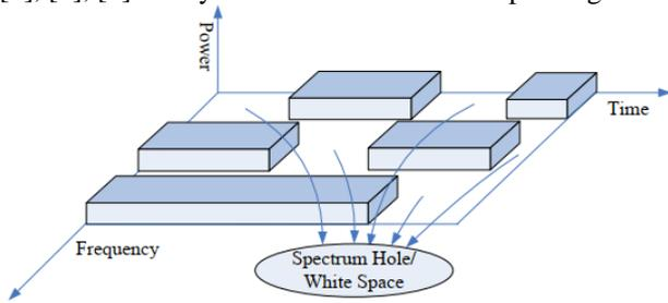
Fig.2 Spectrum Hole Concept
