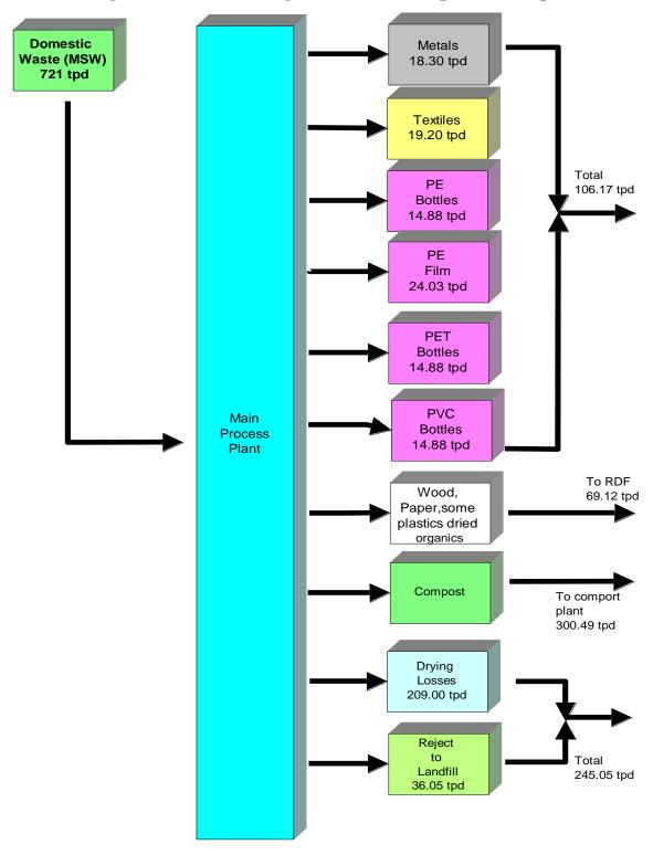
Integrated Waste Management Plant – Inputs & Outputs.
