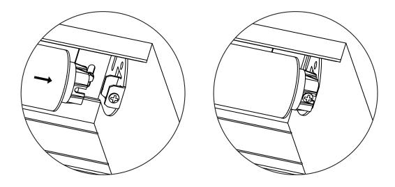
Depress the spring loaded idler by pressing the shade towards the idler, and install the EDU side of the shade onto its bracket.
