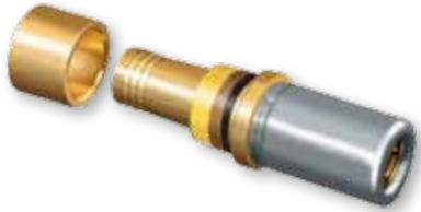
These #12 contacts accept 50 ohm and 75 ohm coaxial cable. Inner contact is rated at 1 amp, the outer contact 12 amps. DWV rating is 1000 Vac rms sea level, 250 Vac at 50,000 feet. Contacts are packaged individually and shipped unassembled with instruction sheet. One contact consists of outer contact, fluorocarbon dielectric, inner contact and shield crimp sleeve. Inner and outer contacts are gold-plated copper alloy. Approved to SAE AS39029. 5000 megohm insulation resistance.
