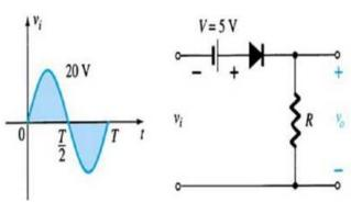
Since the diode is on because of the 5v battery
