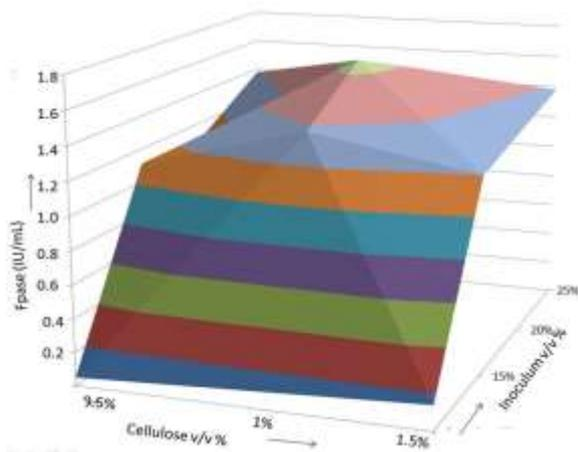
Fig. 1. Response surface curve for the optimization of submerged fermentation for cellulase production
