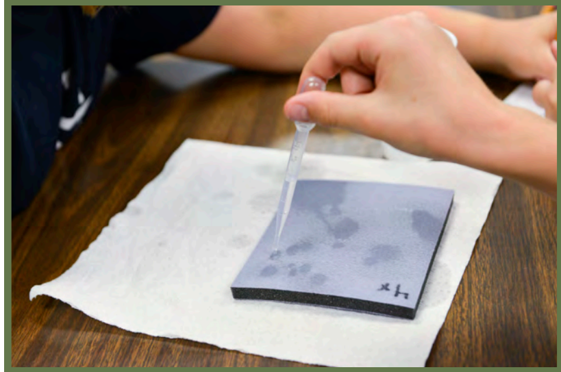
The experiments on the 3M fabric involved observing and measuring water spread across the fabric and water migration through the fabric.
