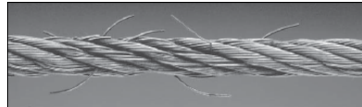
Cable with Broken Wires
