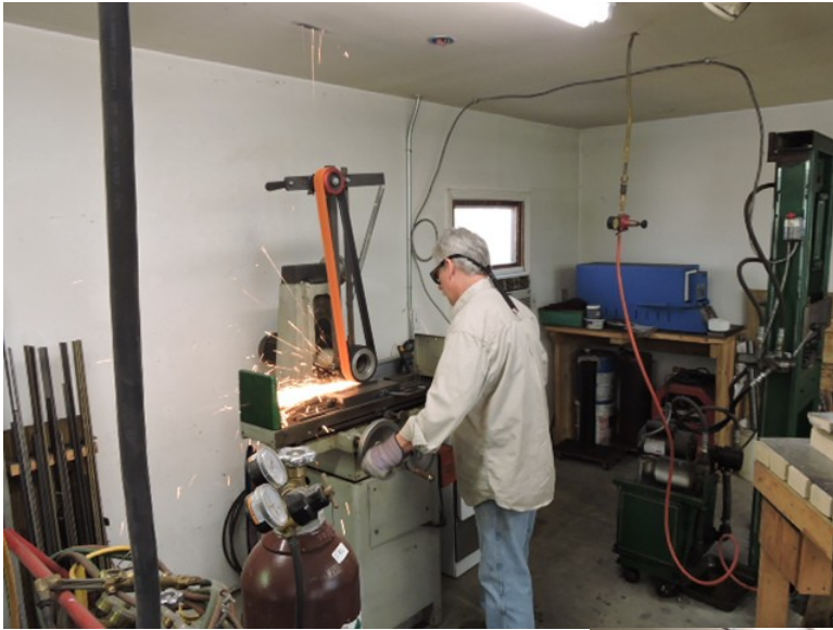
Surface grinding the steel to be all shiny and clean.
