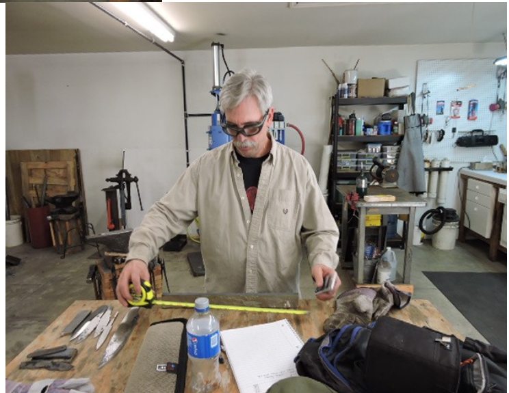
Measuring the billet to get equal cuts for the next stack.
