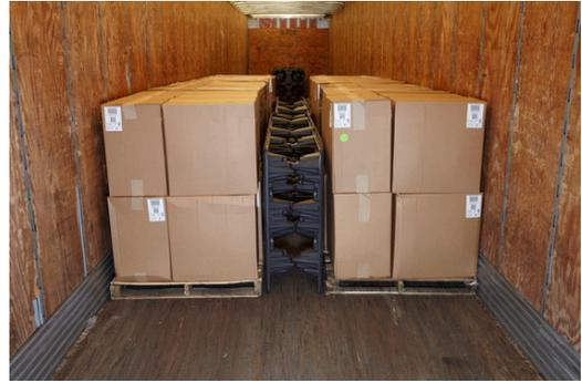
Paylode's Bulkhead Spacers measure 36"Wx48"Lx16"H and are made from 100 percent recycled materials. At end-of-life, Paylode will buy them back to be recycled again, making Bulkhead Spacers a true cradle-to-grave solution.
