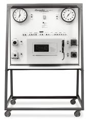
The **Model H-MCP-3A** includes a Synchronous Indicating Clock, Minute Impulse Clock, AC Vibrating Bell, DC Vibrating Bell, AC Singlestroke Chime, DC Singlestroke Chime, AC Remote Buzzer and Master Time Center.
