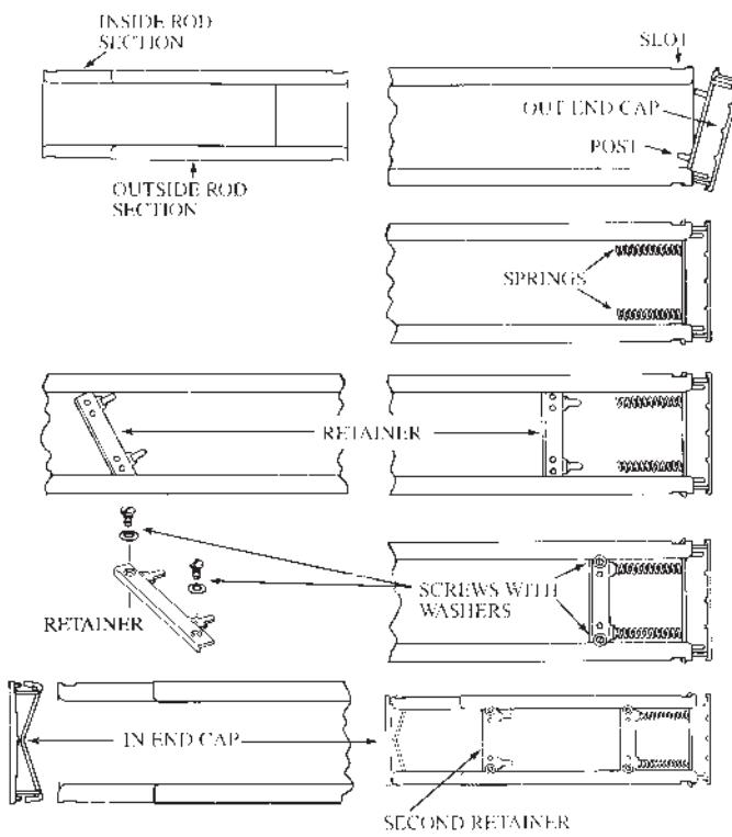
**CAUTION:** For safe and easy assembly, work with rod face down on a flat surface.
