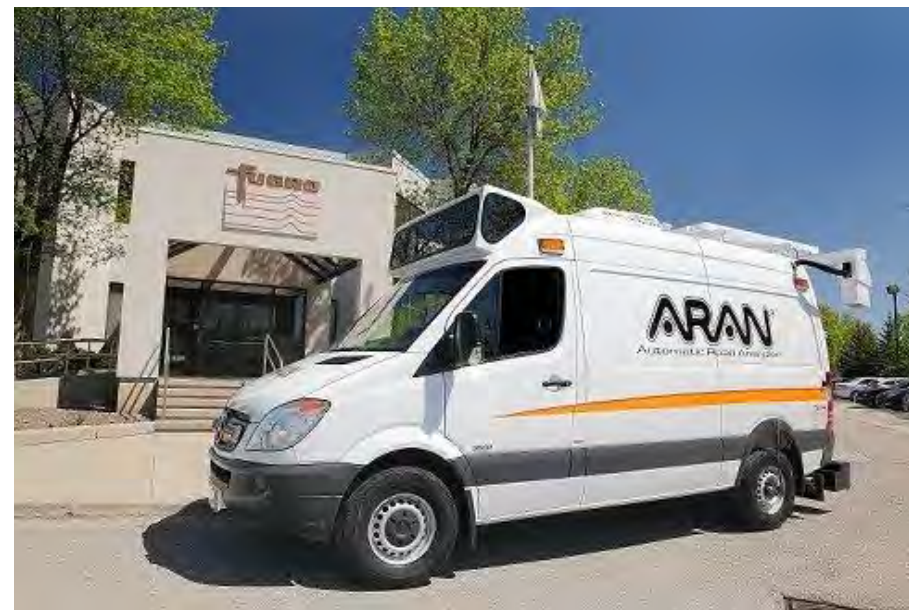
Figure 1: Automatic Road Analyzer (ARAN) - The van is outfitted with an array of sensors and cameras that automatically collect data about the road.
