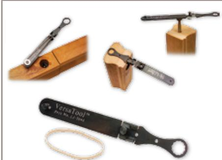
**LJ-3044 VersaTool™** — Locates holes as well as starts and tightens hex nuts onto rail bolts. Drives 5/16" rail bolts and tightens 1/2" hex nuts. Also used to locate 1/4" pilot hole on handrails & rail drops for attaching to Conect-A-Kit® handrail fittings.
