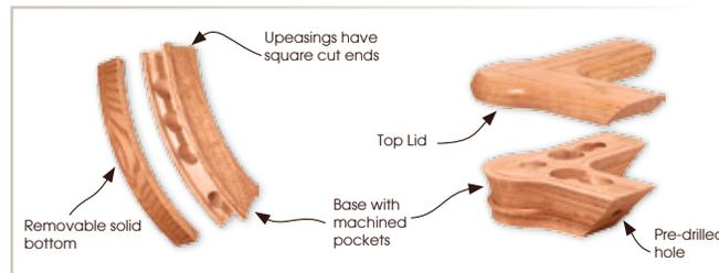
All of the Conect-A-Kit® fittings have a base with machined pockets and a removable top lid (or bottom) for easy installation. All assembly hardware is concealed within the base of each fitting.
