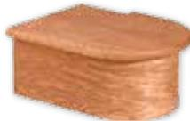
A false end step is used when a volute or turnout is utilized at the bottom of the stairway. Each kit includes cove and shoe moulding, and is reversible for right hand and left hand applications.
