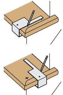
**C-88 Baluster Centerline Tool** — This handy steel tool is used for quick and accurate determination of 1 1/4" (32 mm) and 1 3/4" (44 mm) baluster centerlines on the treads of open tread stairways.
