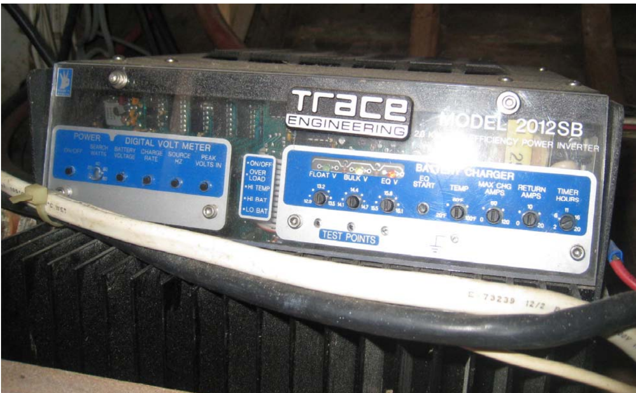
The battery charger appears to have the capability to be manually adjusted. "Boat Name" Surveyed by Island Marine Group, LLC Isle of Palms, SC 29451
