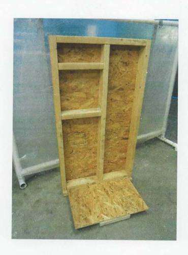
1. Wood stud panels were constructed of standard lumber 2x4's and orient strand board (OSB) to simulate a standard wall cavity of a stick-built house.
