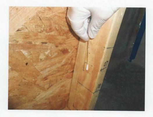
15. Having sample locations pre-marked and pre-numbered allowed for quick and efficient collection of samples. Here, an ATP swab sample was collected from a vertical member after it had been sprayed with Decon 30 and allowed to dry.
