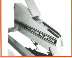
A rubber tyred easily adjustable depth control wheel gives positive depth control. The Paraplow can be easily converted from a three legged to a four legged model by fitting the extension beam, leg and disc assembly.
