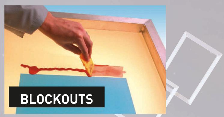
SaatiChem Finish blockouts/screen fillers offer both high performance and user friendliness. Finish blockouts contain no solvents and provide increased filling power. All have pleasant-smelling formulations and are non-hazardous and biodegradable. Finish blockouts spread smooth and uniformly for optimum drying and filling. Use to cover open mesh areas and pinholes.
