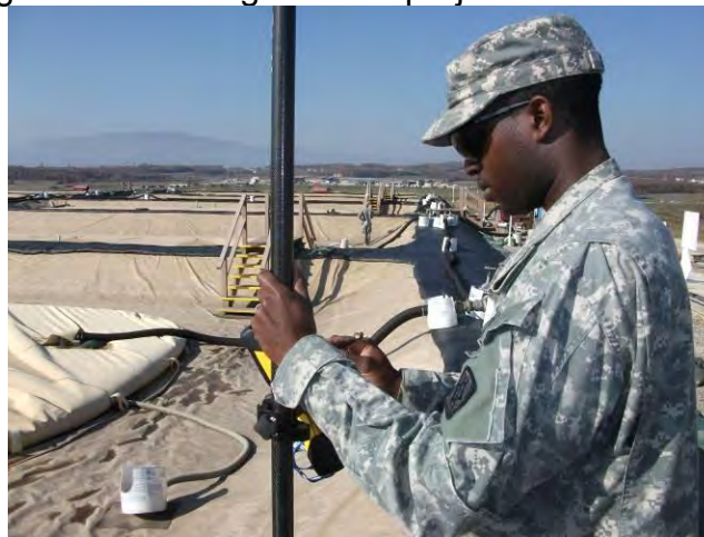
Spc. Darius Cooper, a technical engineer with 18 th Engineer Brigade from Portsmouth, Va., surveys a bulk fuel farm Oct. 23 at Camp Bondsteel, Kosovo, to help the Director of Public Works come up with a better plan to help store fuel. The results of the mission gave the DPW a way of accurately accounting for the fuel contained or lost. (Photo by Staff Sgt. Robert Owens, 18 th Engineer Brigade)
