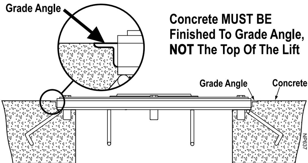
**Owner: Your Installer Is Responsible For The Concrete Floor Being Finished To Grade Angle, NOT To The Top Of The Lift. Failure To Comply Will Void Warranty**
