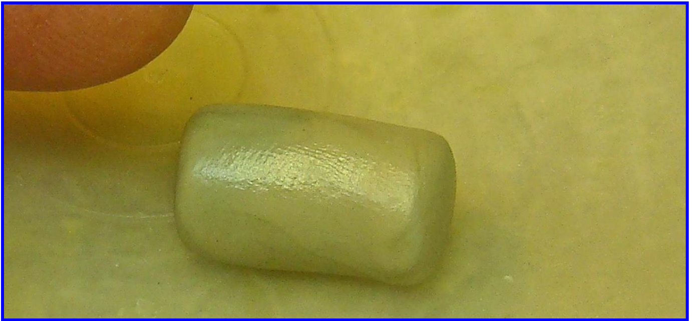
Figure 006 – Kneading the Epoxy into a Cylinder
