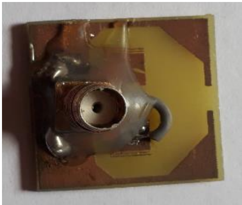
Figure 3: fabrication of antenna step 3
