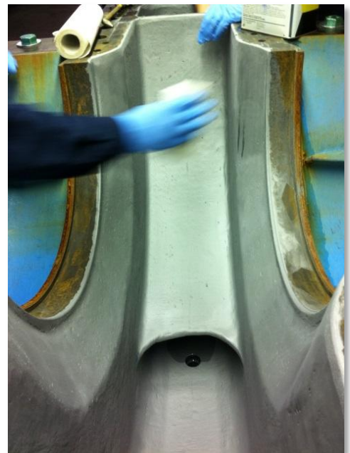
Acetone Wipe – used for final degreasing of surface to be coated
