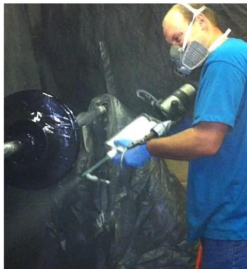
For both small and large jobs, Adiacoat Elastomer Coating can be applied by low pressure spraying.
