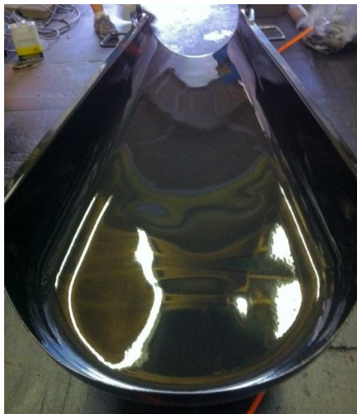
Cement chute coated using casting technique enables repeated coating with uniform coating thickness and improved surface finish
