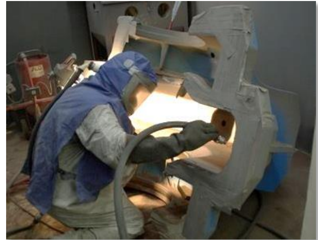
Grit Blasting – preferred method for cleaning and roughing the surface to be coated
