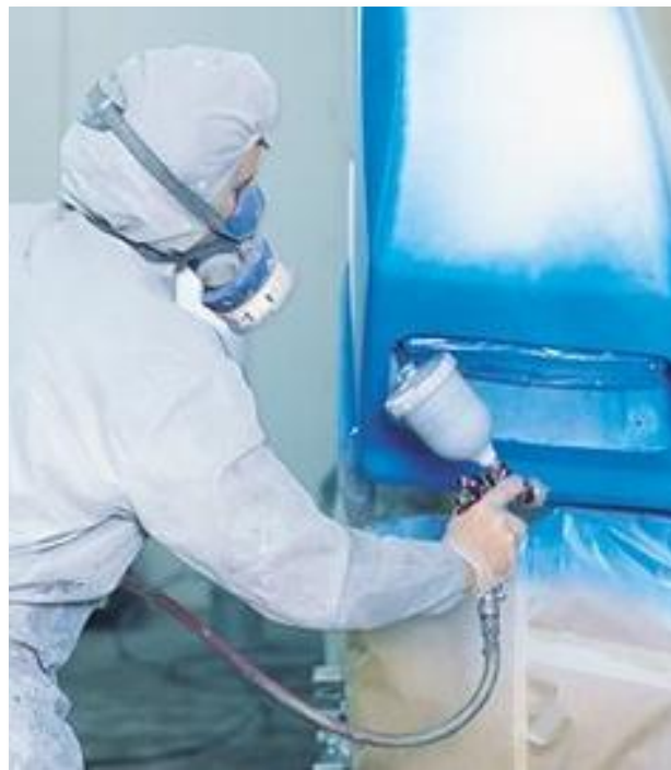
For very large area applications or in cases as shown above (hard to reach areas), HVLP spraying of primer can be used
