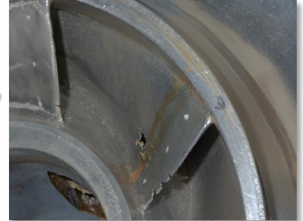
Water pump damage from cavitation and erosion can be prevented or repaired using Adiaccoat Elastomer.
