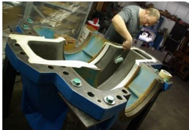
Priming can be done simply by brushing or rolling as shown above.
