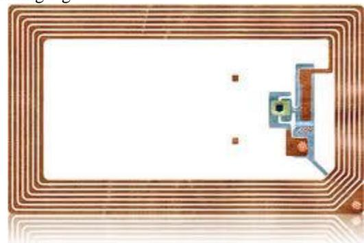
Fig.3: RFID tag inner view
