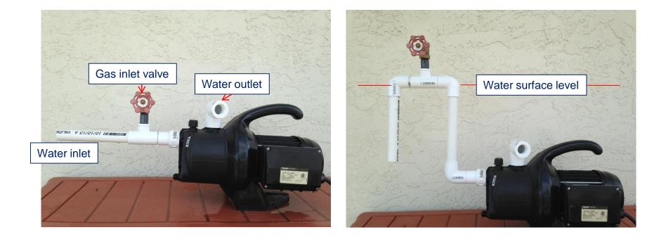
Note : When your water level is higher than the pump location, water static pressure can exceed the negative pressure resulting no suction. In that case, please set the gas inlet point higher that water surface like right picture.
