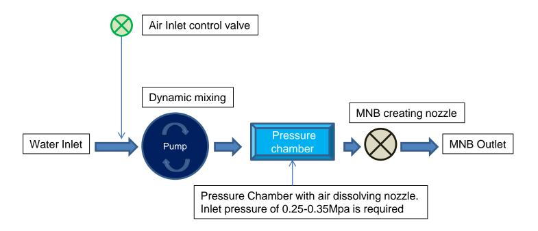
Water and air is mixed in the pump and move to pressure chamber. The process of dissolving gas happens in the chamber. The water after the chamber have oversaturated air and MNB is created by the nozzle when the water get released to atmosphere pressure.
