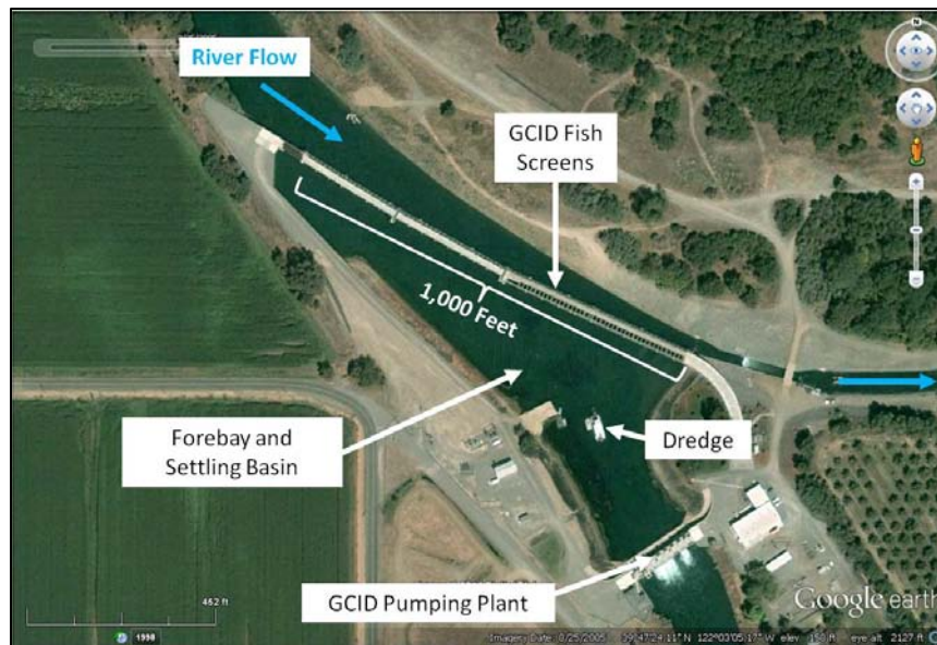
Figure 19. Aerial photograph of the GCID fish screens showing the large forebay behind the fish screens and upstream of the GCID pumping plant.
