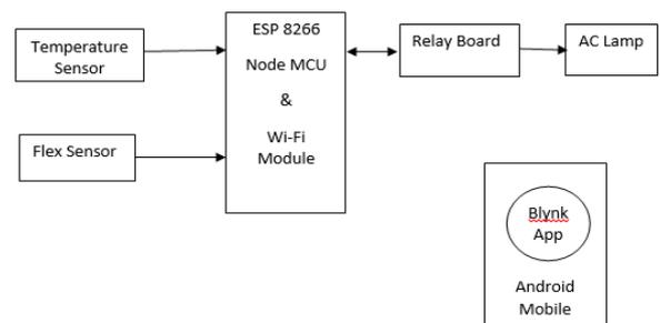
Fig 1: Block diagram of Cloud-Based Remote Monitoring Applications with WSN
