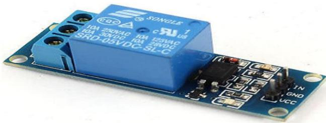
Fig 6: Relay Board
