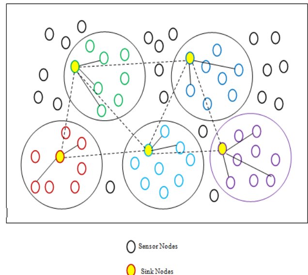
Fig.1: System model of proposed efficient sink repositioning technique (ESR)
