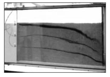
Drainage (Seepage) Flow Through the Wall of an Open Trench
