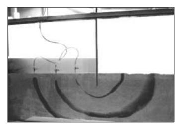
**Purpose:** To 1) demonstrate the lines of flow (path of percolation) under wall pilings (footings), 2) determine the rate of seepage, and 3) allow for the construction of equipotential lines (i.e. develop a "flow net").
