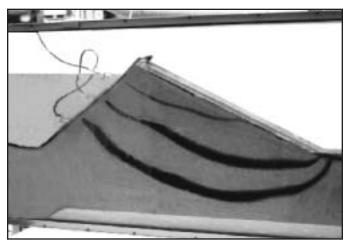
**Purpose:** To 1) demonstrate the flow lines through a sloped earth embankment, 2) determine the rate of seepage, and 3) allow for the construction of equipotential lines (i.e. develop a "flow net").
