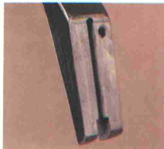
B. The back of each limb is machined with a locator pinhole and limb microgroove alignment key way. The locator pin and pinhole match for perfect fit and positive limb alignment.
