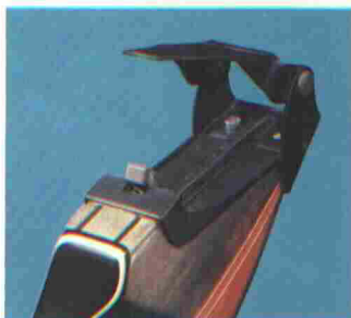
C. Opened handle socket showing limb alignment key and stop screw.
