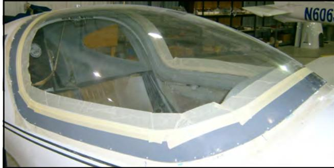
**Note:** Canopy frame must be fitted to the fuselage, canopy tip up support arms installed, overhead latch installed, cockpit side location tabs installed, and gas strut ball ends in place. **This task is best done before the firewall and pedal assemblies are in place, this allows you to crawl in the front and clean up the glue which will come out around the flange.**
