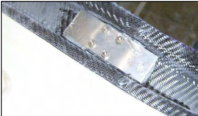
6. The gap between the frame and fuselage should be about 1/16”.
