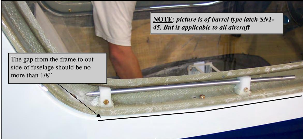
3. The gap between the frame and the fuselage from 10" either side of center should be 1/8". This is where when the canopy opens the frame rotates slightly to the fuselage instead of up and away.
