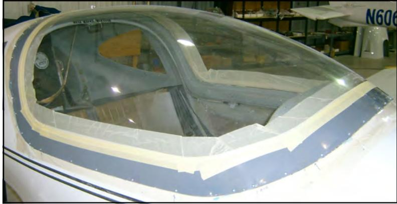
30. Use the left over skins to make a part to finish out over the canopy latch. There is no measurements just need to make a skin to fit.
