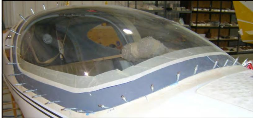
Prep Fuselage with packaging tape so the frame will not bond to the fuselage!!!
