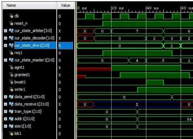
Fig. 3. Simulation results of ASB Non-Sequential Write Transfer Cycle
