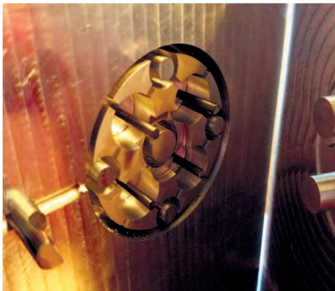
**Made just a few months ago, this is the first low-volume injection mold insert that Nonspec had produced to test the mold design of one of its lower limb plates.**
